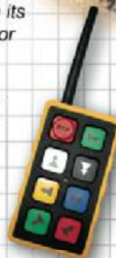
Mini V2 with two-single-speed buttons, start and stop
